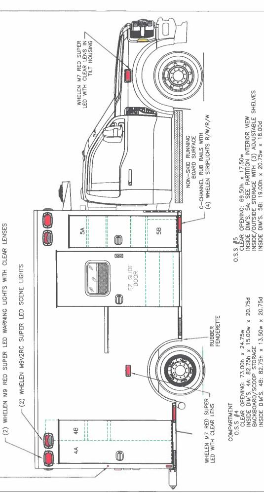
THIS DRAWING IS FOR REPRESENTATIONAL PURPOSES ONLY. DETAILS ARE CONCEPTUAL AND ARE SUBJECT TO CHANGE DURING DESIGN AND CONSTRUCTION DIMENSIONS ARE APPROXIMATE UNLESS NOTED OTHERWISE TO MEET A SPECIFIC CUSTOMER NEED. INSIDE DIM'S. 4B: 82.75h × 13.50w × 20.75d (2) ADJUSTABLE SHELVES WITH INSIDE/OUTSIDE ACCESS
