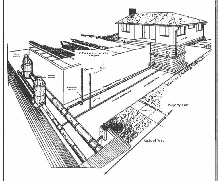
Storm Sewer System - is everything outside of the house, downspouts, driveway drains and rear yard/surface drains. The storm line is trapped at the test tee.
